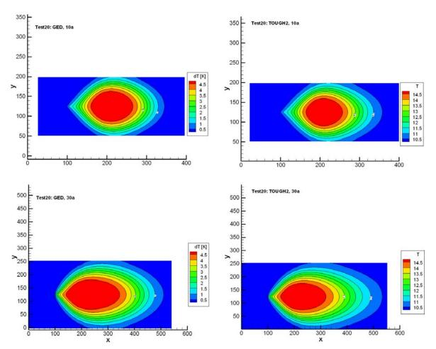
Figure 4: Comparison of results: left GED, right TOUGH2, on top after 10 years, on bottom after 30 years of operation.
