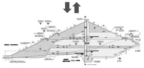
Optimized embankment zoning to increase dam safety and stability during seismic events
